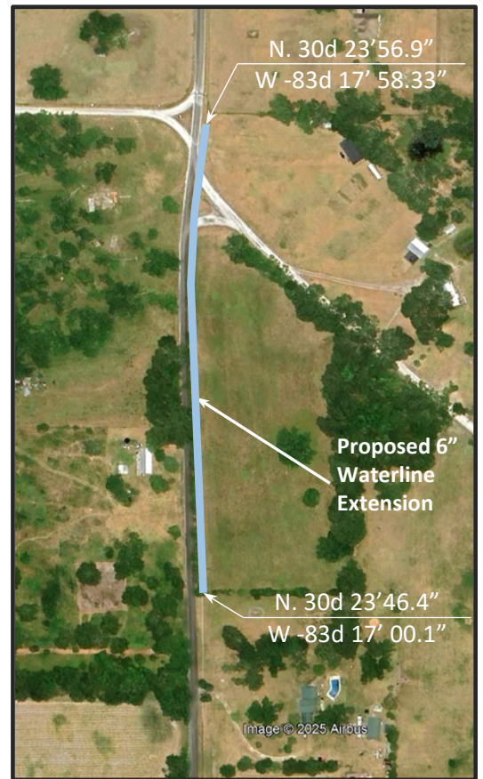
Service Area 2 Proposed 6" Water Main Extension
